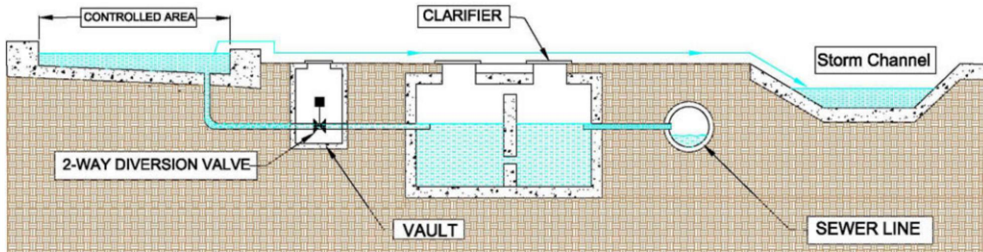
Stormwater Diversion by 3-way butterfly or ball valve located downstream of clarifier.
