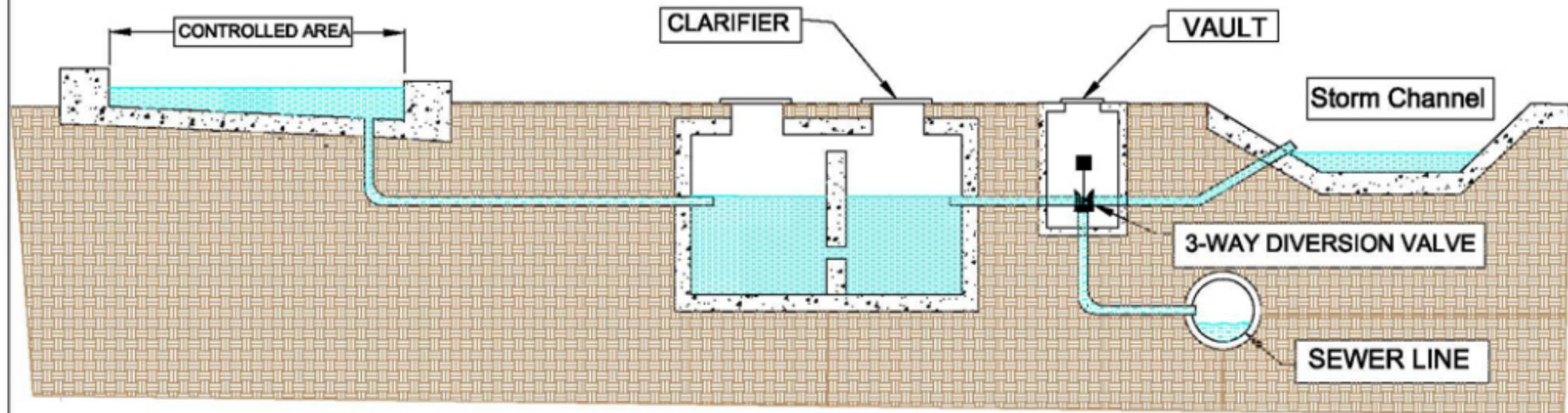
Stormwater Diversion by 3-way butterfly or ball valve located upstream of clarifier.
